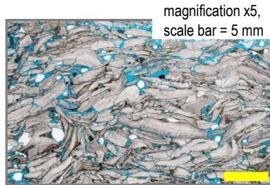
Rock type RT-1: no clay, no micrite, developed intergranular porosity
