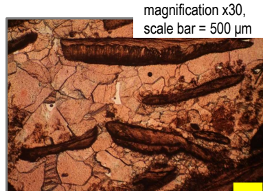
Rock type RT-3: no clay, prevalent micrite and calcite cementation, no intergranular porosity
